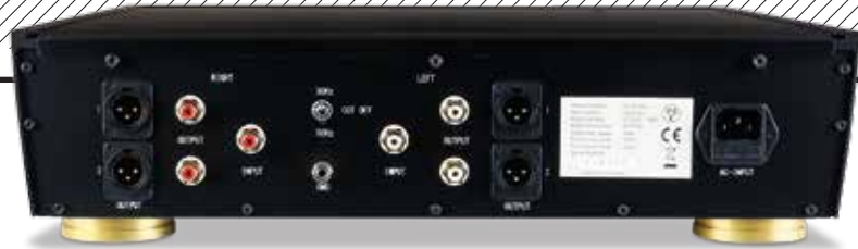
ABOVE: Rear view of the DS-W3's PSU/equaliser. The pick-up's internal 5V LED is powered via the R- and L- pins while the output is returned via R+ and L+, through the 'input' RCAs. The equalised outs, on RCAs and XLRs, are filtered at either 30Hz or 50Hz
